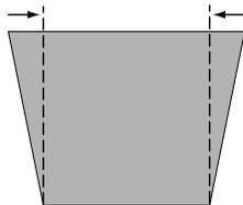
Reduce the lower width with KEY STONE ▼ button or POINT DOWN button.
