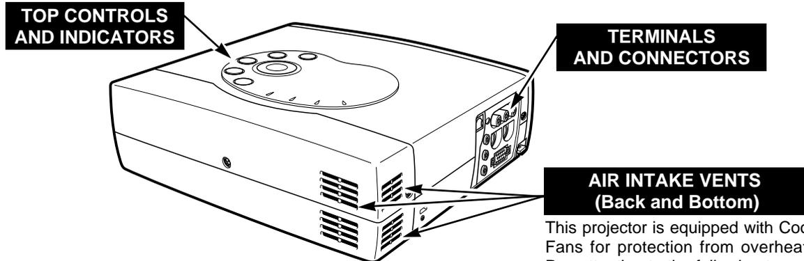
This projector is equipped with Cooling Fans for protection from overheating. Pay attention to the following to ensure proper ventilation and avoid a possible risk of fire and malfunction.
