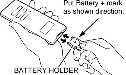
**3** Install battery and Battery Holder into Remote Control Unit.
