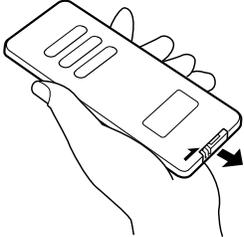
**2** Replace with new battery. Install with battery (+),(-) marks properly.
